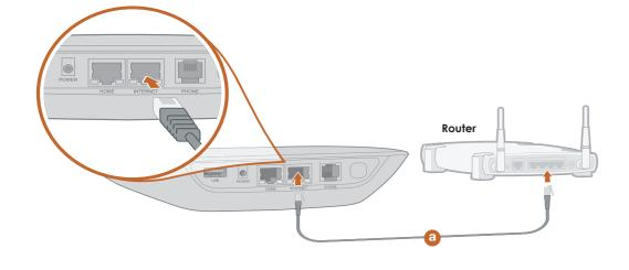
Connect the Ooma Telo to your Router Using the included Ethernet cable (a), connect the
